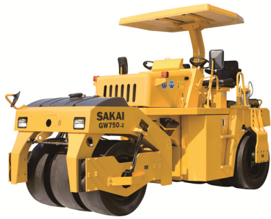
VIBRATORY PNEUMATIC TIRED ROLLER GW750 9,240Kg(20,370Lb)
