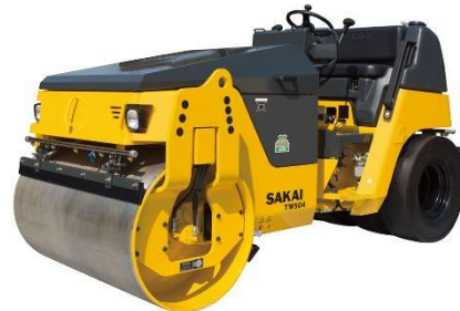
VIBRATORY DOUBLE DRUM ROLLER TW504 3,620Kg (7,980Lb)
