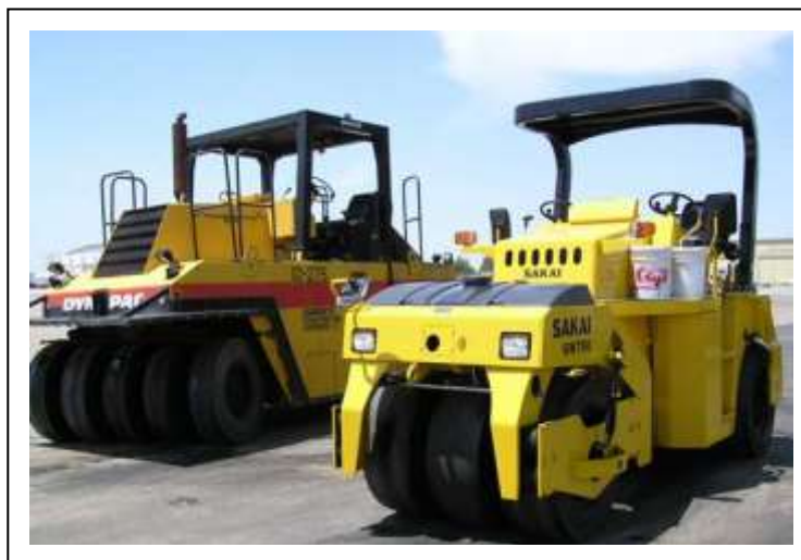
FIGURE.1 Conventional SPT static roller (left); fourth generation VPT roller (right).
