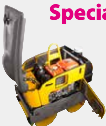
One-touch open covers for easy maintenance
