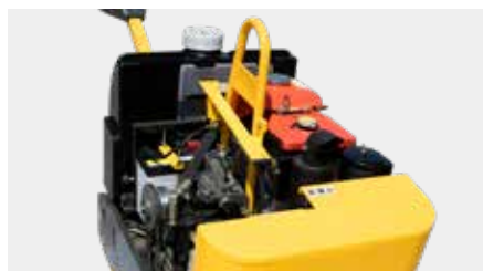
Full-open type cover for easy maintenance
