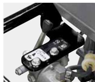
One throttle lever (Engine-off, Fuel-off, Throttle adjustment)
