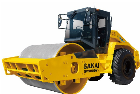
VIBRATORY SINGLE DRUM ROLLER SV900DV 20,030Kg (44,460Lb)
