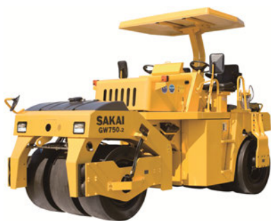
VIBRATORY PNEUMATIC TIRED ROLLER GW750-2 9,040Kg (19,930Lb)
