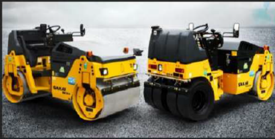
Tandem Roller (left)/Combined Roller (right)
