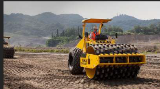
Vibratory Single Drum Roller for large-scale earthworks
