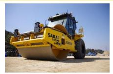
Conducted a rental for an autonomous roller (automatic operation) to Tamashima-Kasaoka road improvement project in Okayama Prefecture. This is the second rental project after Shin-Maruyama Dam in Gifu Prefecture. This is the first time in Japan to utilize an autonomous roller for road construction projects.
