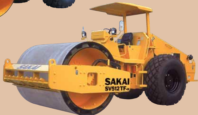
SV512TF-H Padfoot drum with removable smooth drum shell Gross weights 13 ton (28,660 lb)
